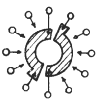
WAFER SWITCH (EXAMPLE) VIEWED FROM THE REAR
