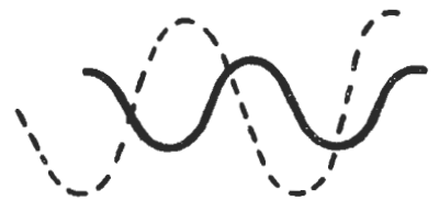
DEMODULATED SIGNAL COMPLETE LOSS OF INTELLIGIBILITY
