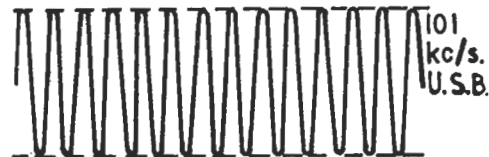
SINGLE TONE OUTPUT AFTER FILTERING OUT THE L.S.B. THIS IS THE S.S.B. SIGNAL THAT IS TO BE TRANSMITTED.
