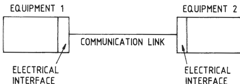
FIG 8.1 ESSENTIAL ELEMENTS OF A COMMUNICATION LINK
