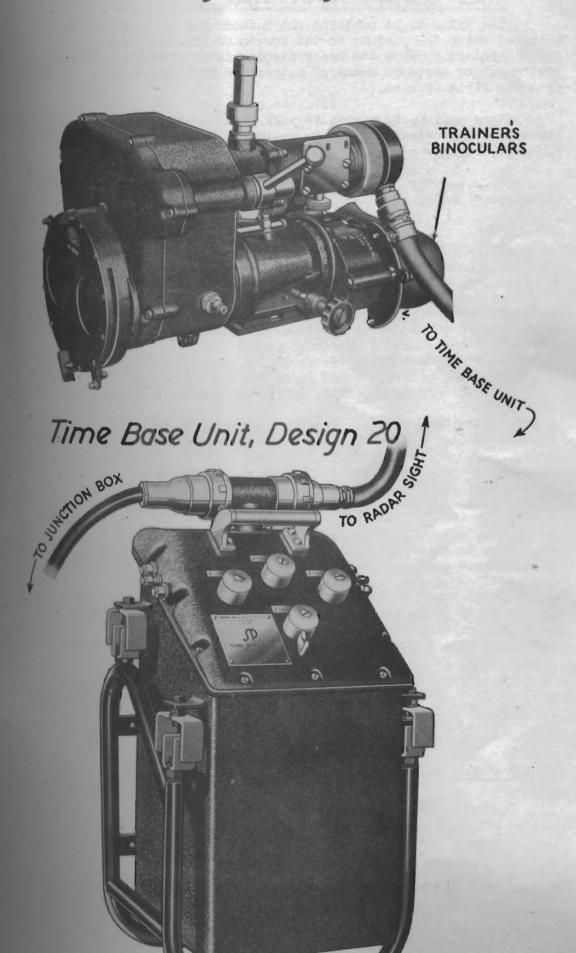
have been taken to keep the unit dry and watertight; all the control knobs have their own integral air seals and provision is made for attaching a dessicator and pump to pass dry air through the unit.
